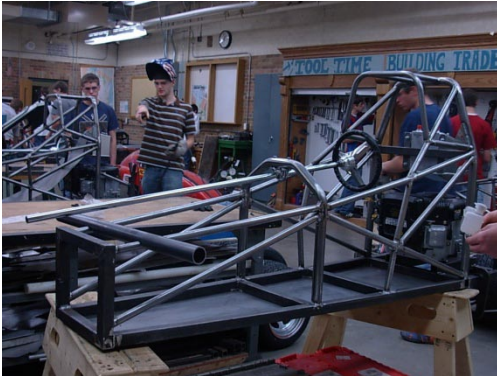
The finished chassis with the floor installed. The steering wheel is being ready to be installed.
