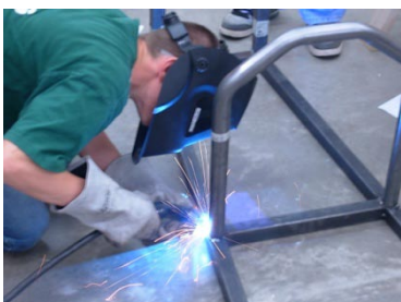
Jim welding the middle roll bar to the chassis.
