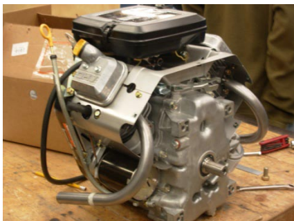
Our vertical shaft engine with the beginnings of the exhaust system installed.
